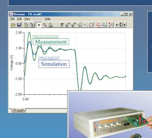
Using TINALab II with DesignSoft's popular circuit simulation program, gives you the unique capability to have circuit simulation and real time measurements in the same integrated environment. This provides an invaluable tool for troubleshooting and brings your designs to life by comparing simulated and measured results.
