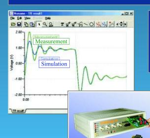
Using TINALab II with **TINA PRO**, DesignSoft's popular circuit simulation program, gives you the unique capability to have circuit simulation and real time measurements in the same integrated environment. This provides an invaluable tool for troubleshooting and brings your designs to life by comparing simulated and measured results.
